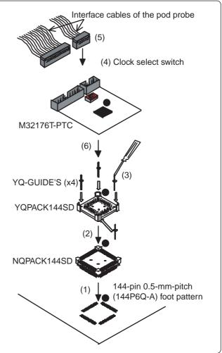
Figure 3 Connection procedure of the M32176T-PTC
